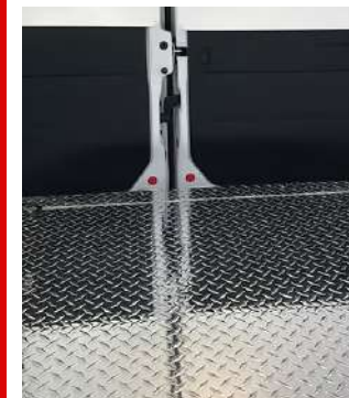
Aluminum floor cut from CNC machine
