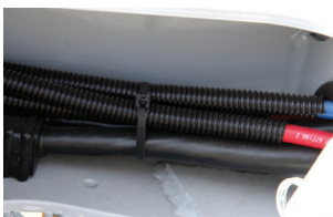
Air and electrical lines protected with Automotive Wire Loom for optimal wire protection
