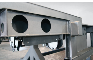
All fabricated steel parts are shot blasted, prime coated before and after fabrication and welding then followed with a zinc rich epoxy primer
